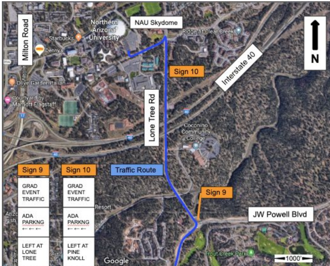
Figure 7: Long-term Traffic Circulation Plan along JW Powell Blvd and Lone Tree Road south of NAU Campus and the NAU Skydome [1].
